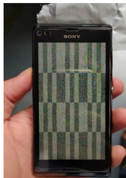
Figure 11: Damage to the phone's display.
