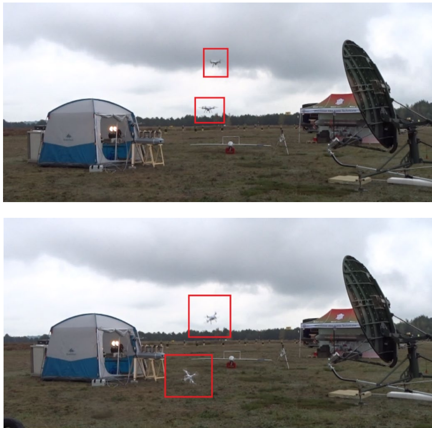
Figure 21: The moment of disabling the Syma UAV by the HPM impulse.
