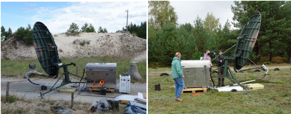
Figure 8: HPM impulse generation setups.
