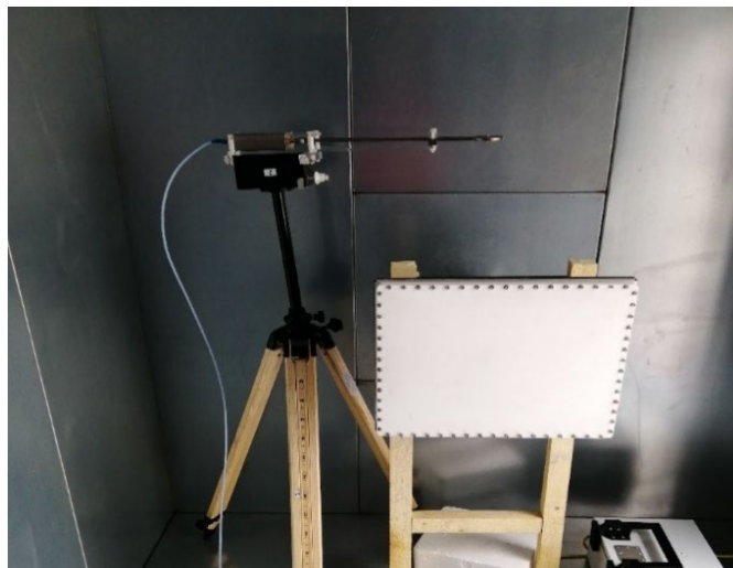
Figure 2: Field intensity measurement system.
