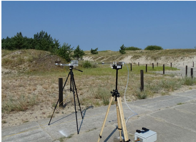
Figure 9: Measured electric field intensity distribution; particular measurement amounted 17.0 kV/m at a distance 23 m.
